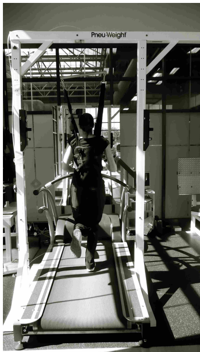
Figure 1. High speed treadmill with body weight support harnessing system
